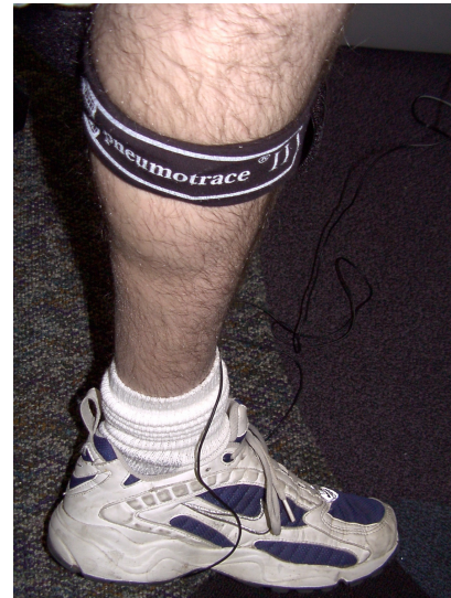
Figure 4: Attachment of the respiratory belt transducer to the calf for leg volume measurement.
