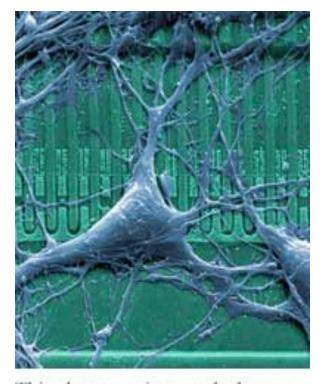
This electron micrograph shows a nerve cell connected to an oxidized silicon chip coated with collagen. The ion current the cell uses for communication flows along the narrow gap between the cell and chip and affects the silicon electrons' flow.
